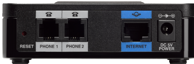
Figure 2. Ports on Cisco SPA112 ATA 2 Port Adapter
